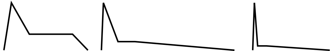
Figure 4.7 ADSR shapes for a “trumpet” envelope, a “piano” envelope, and a “kick drum” envelope.
