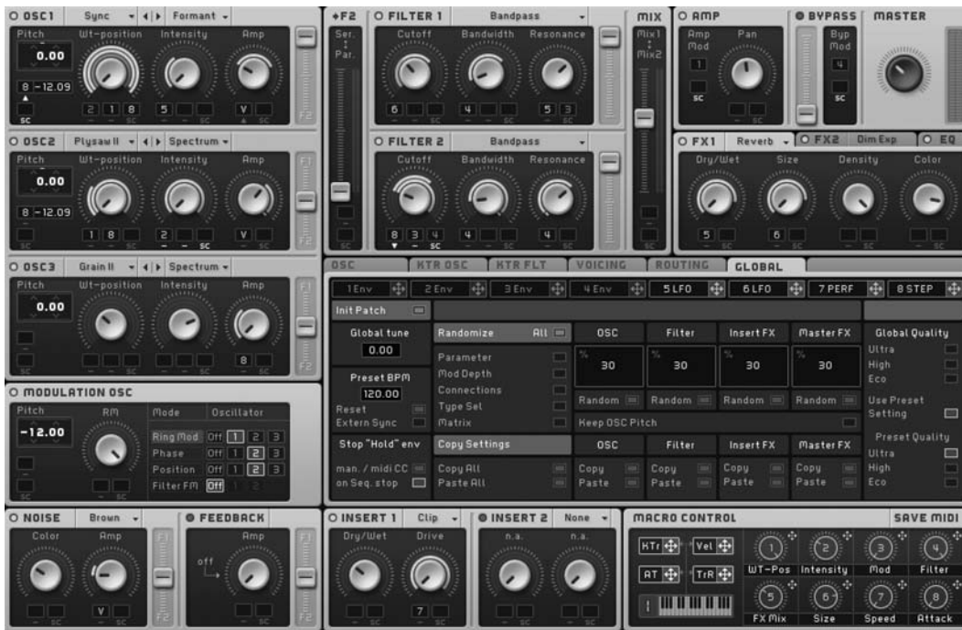
Figure 1.19 Native Instruments’ Massive softsynth provides a huge array of sound creation and shaping tools and can run on its own as a stand-alone instrument or as a plug-in inside of most DAWs. Massive can also map the various knobs and other physical controls from an external hardware controller to the instrument’s many functions via the Macro Control panel located at the bottom-right of the softsynth’s window.
